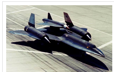
The D-21 mounted on the back of the M-21. Note the intake cover on the drone, which was used on early flights.
