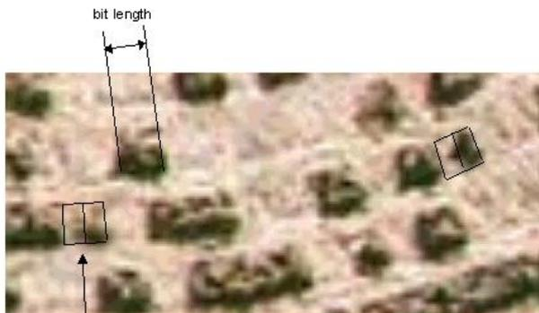
byte delimiter (half bit down, half bit up)
