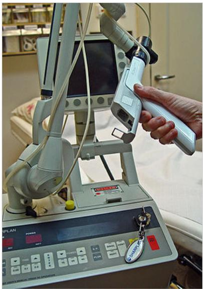
A 40 watt CO<sub>2</sub> laser used for podiatry
